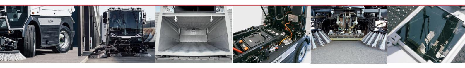
4 wheel steering 3rd brush 5.6 m³ Hopper 137 kWh Bucher Battery Pack Wide suction intake Floor glas panel
